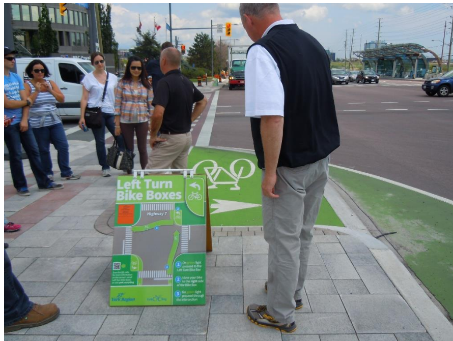
Figure 7.1 Demonstration of left-turn bike boxes at a signalized intersection to improve cyclist safety and navigation (York Region).
